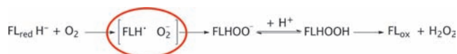
Figure 1. Mechanism of reaction of reduced flavin with oxygen. It has been proposed that stabilizing the superoxide-semiquinone pair (circled in red) allows rapid reaction with \text{O}_2 .
